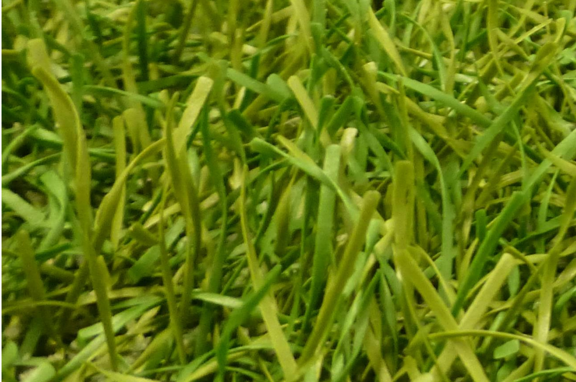
Fig. 10: FieldTurf Quattro after 200.000 Cycles at the Lisport tester
