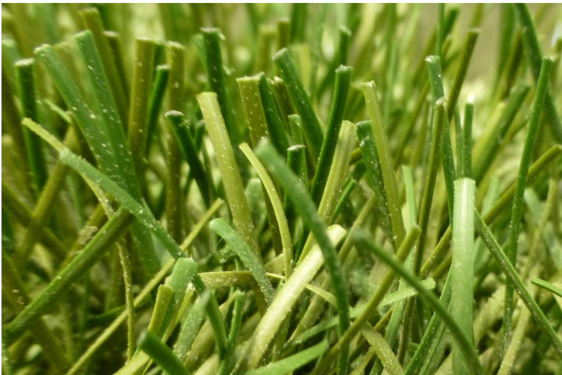
Fig. 7: FieldTurf Quattro after 100.000 Cycles at the Lisport tester
