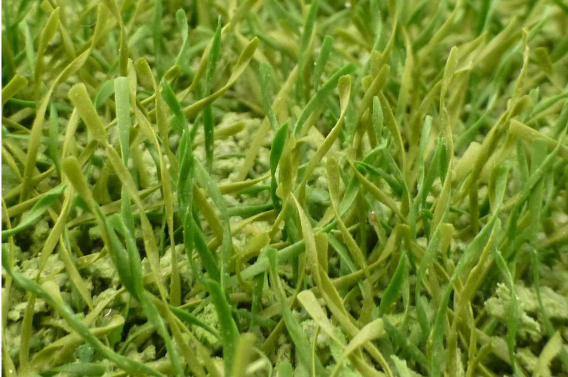
Fig. 12: FieldTurf Quattro after 250.000 Cycles at the Lisport tester
