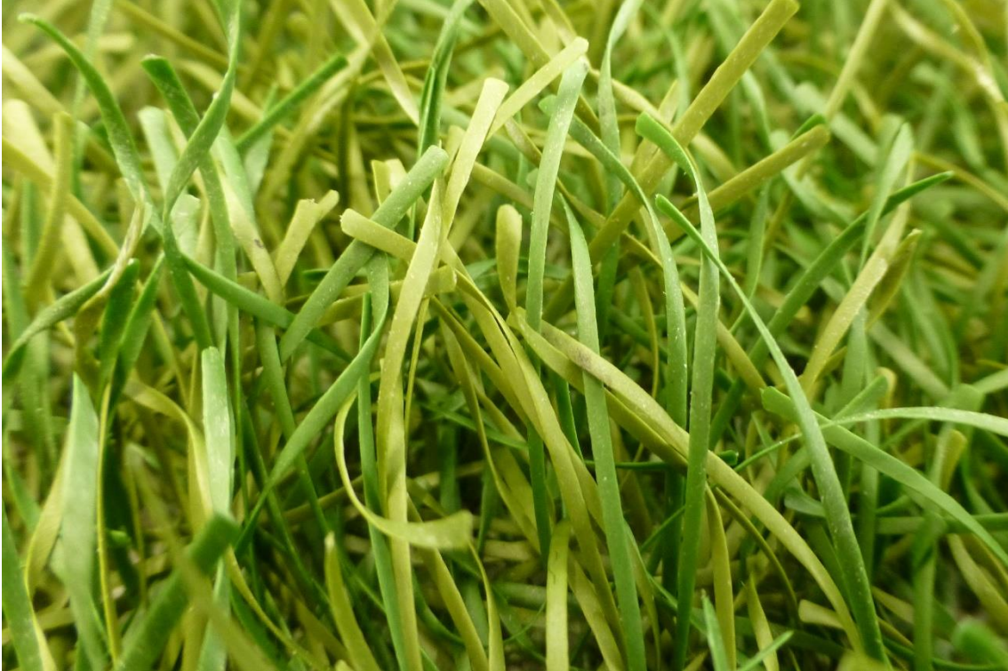
Fig. 8: FieldTurf Quattro after 150.000 Cycles at the Lisport tester
