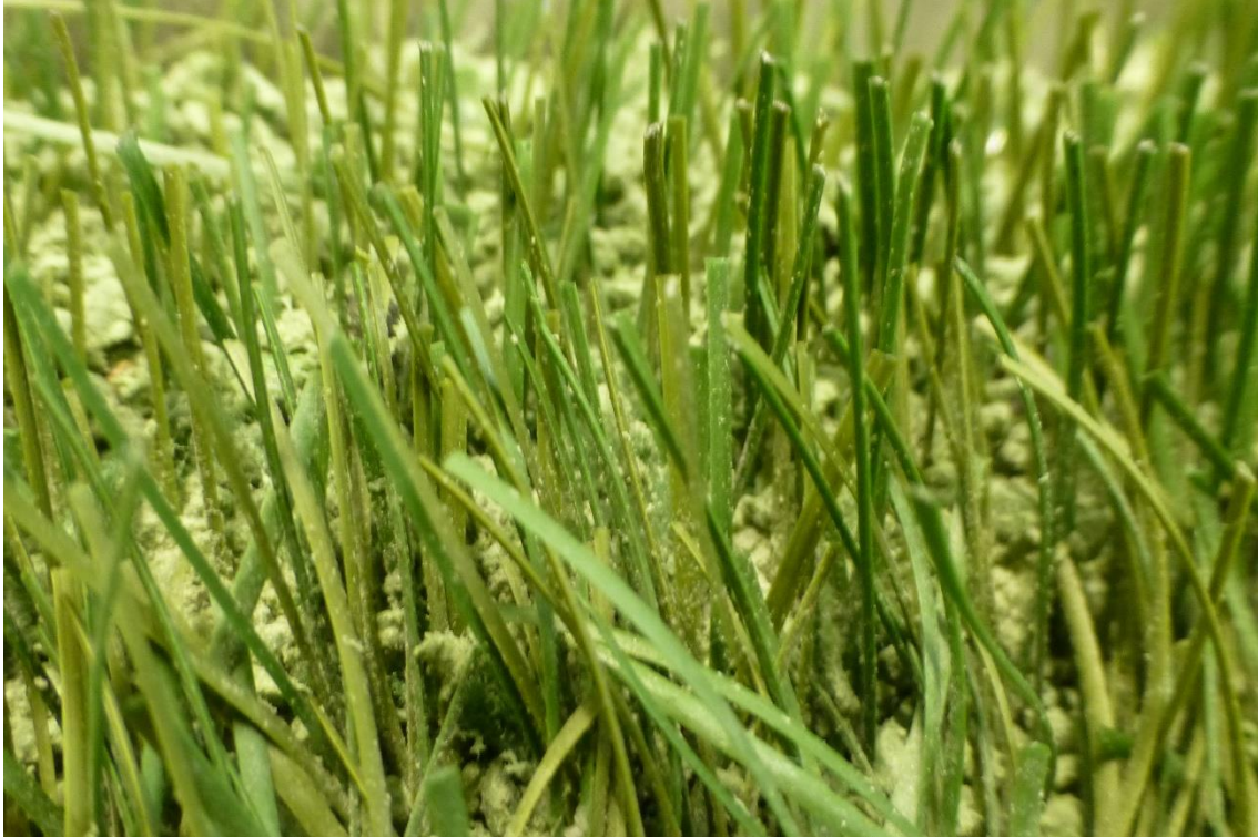
Fig. 6: FieldTurf Quattro after 100.000 Cycles at the Lisport tester
