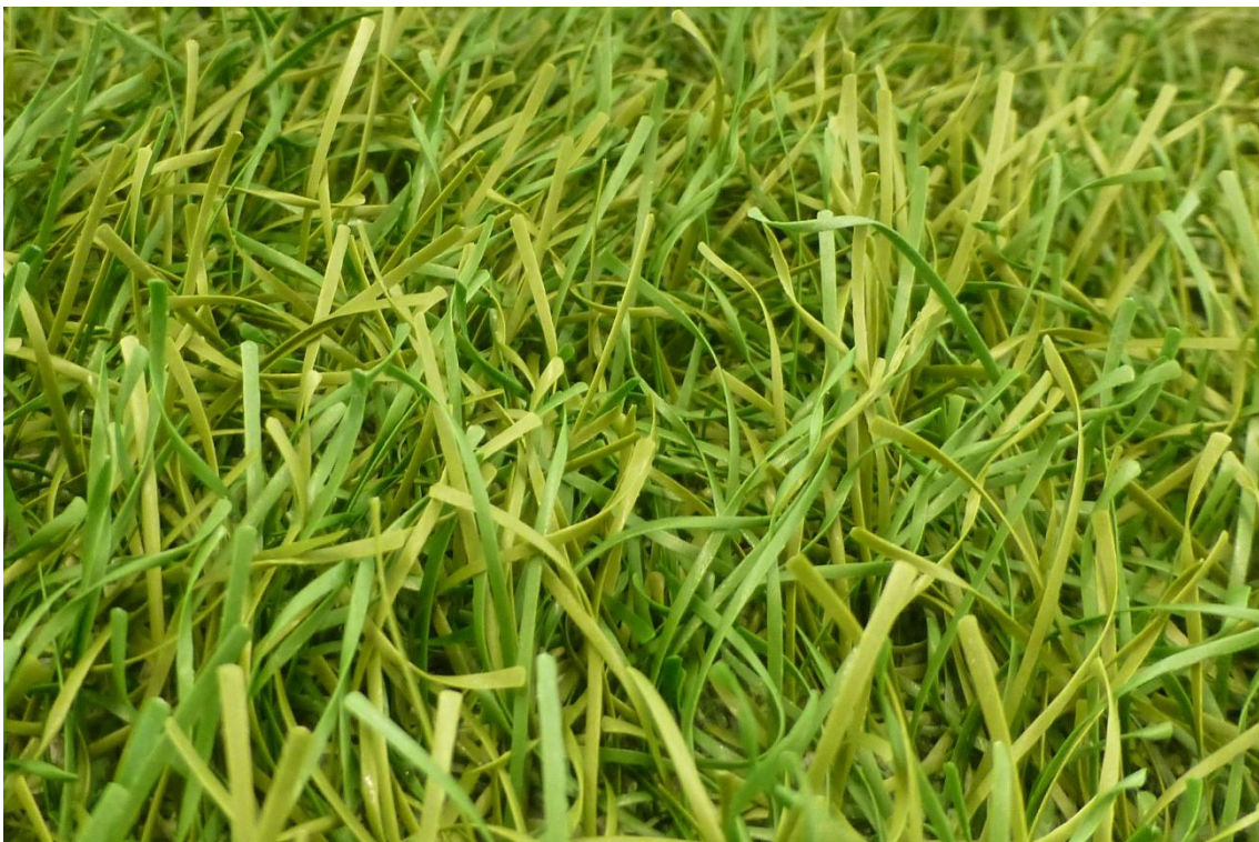
Fig. 9: FieldTurf Quattro after 150.000 Cycles at the Lisport tester
