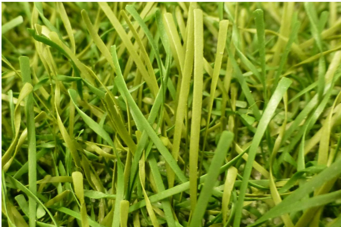
Fig. 11: FieldTurf Quattro after 200.000 Cycles at the Lisport tester
