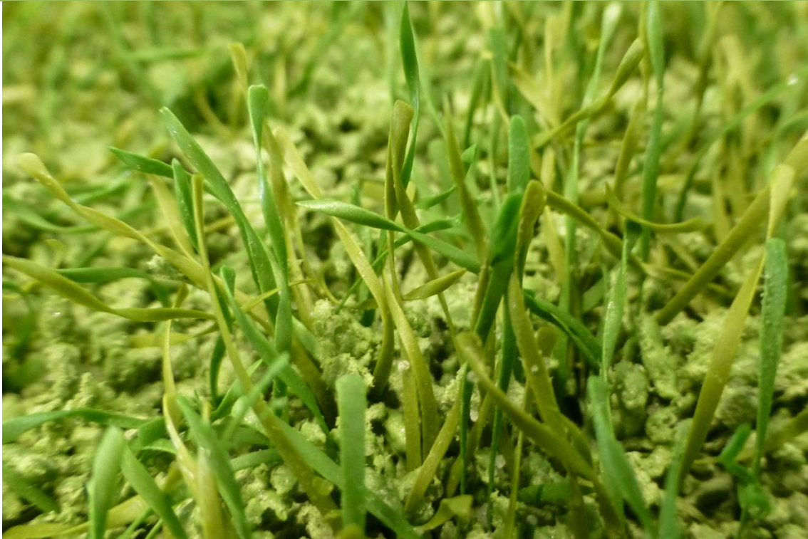
Fig. 14: FieldTurf Quattro after 300.000 Cycles at the Lisport tester
