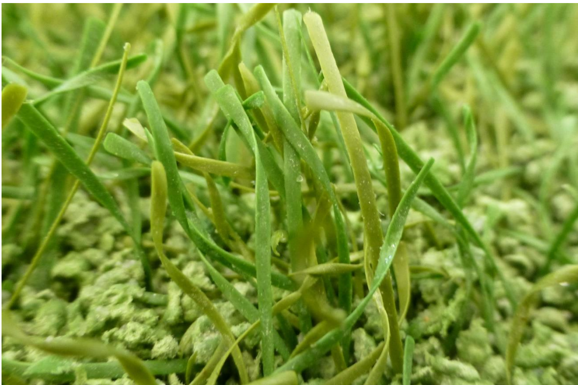
Fig. 13: FieldTurf Quattro after 250.000 Cycles at the Lisport tester
