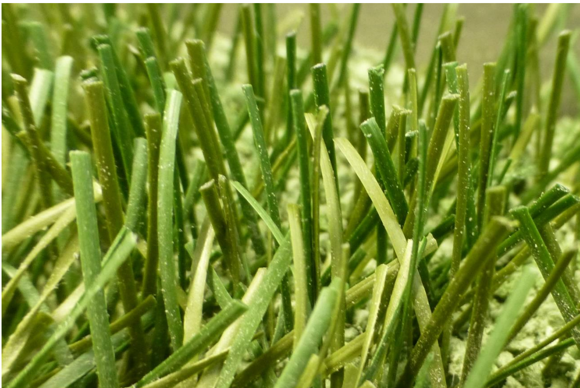
Fig. 5: FieldTurf Quattro after 50.000 Cycles at the Lisport tester
