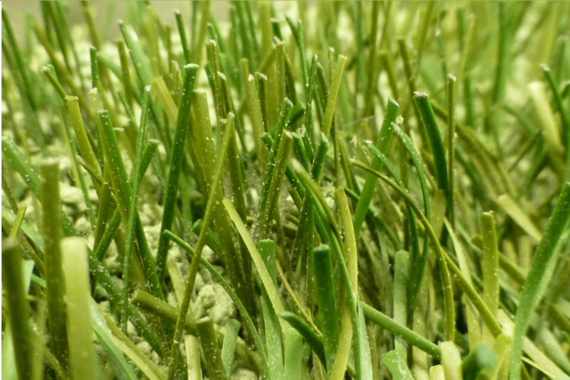
Fig. 4: FieldTurf Quattro after 50.000 Cycles at the Lisport tester
