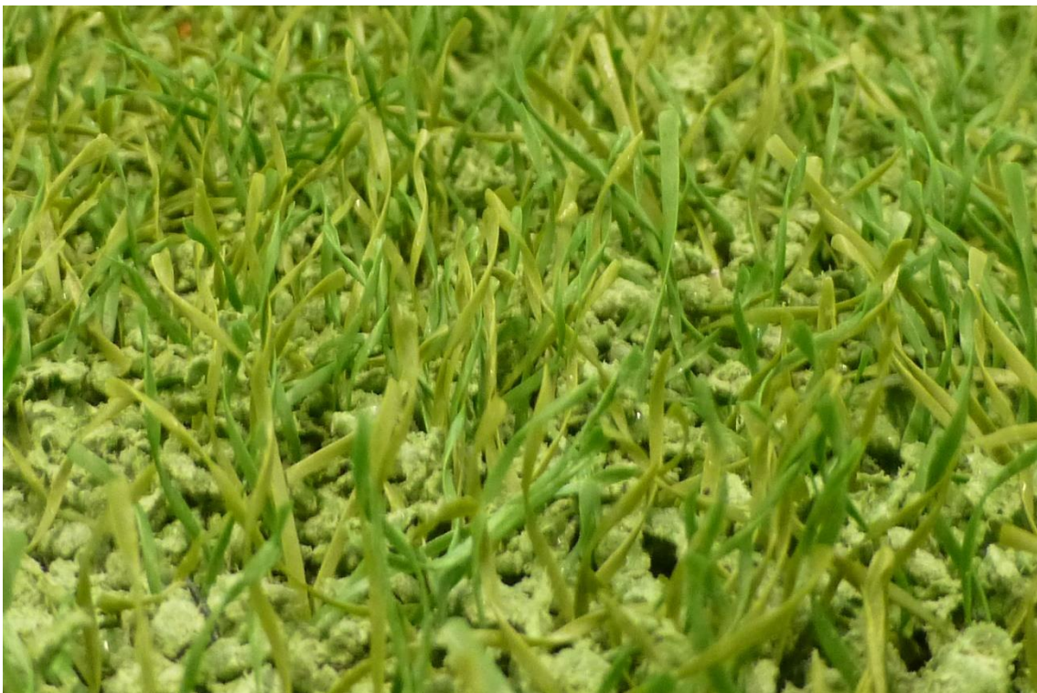
Fig. 15: FieldTurf Quattro after 300.000 Cycles at the Lisport tester
